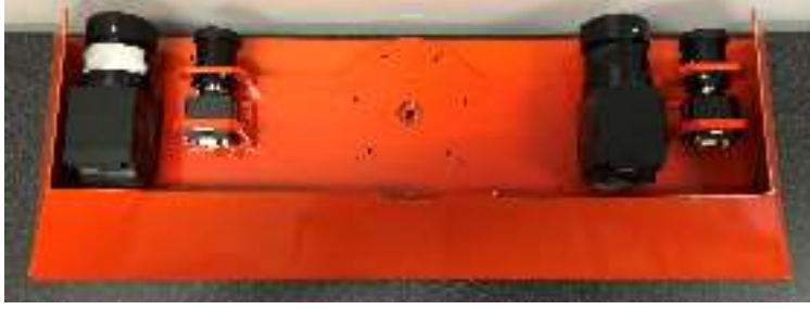
Fig. 2 Low-resolution EO cameras and IR cameras mounted for the first experiment
