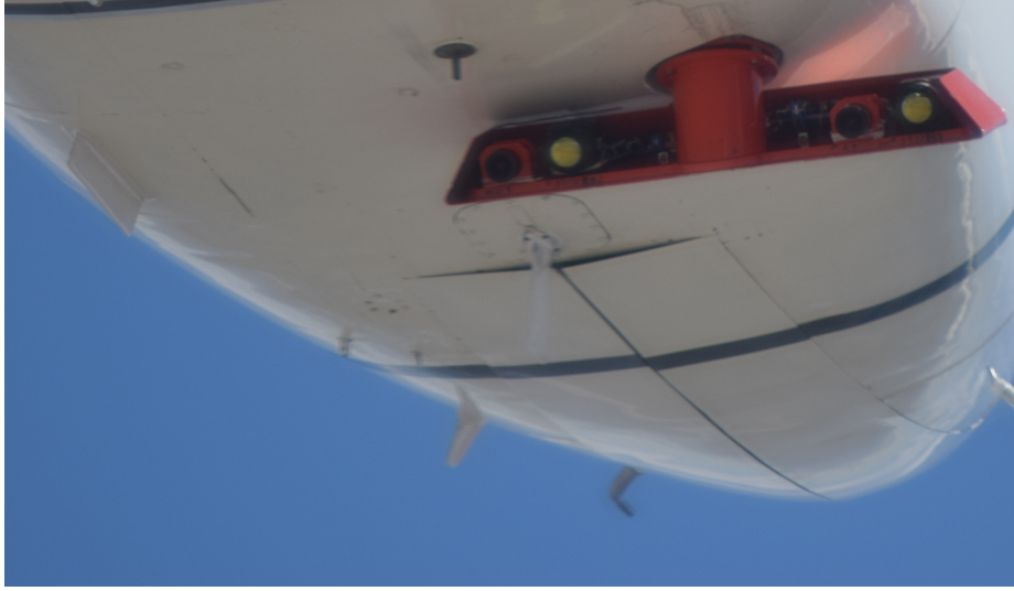
Fig. 3: Reference image of stereo EO and IR cameras mounted underneath the co-pilot.
